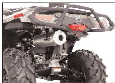
All-out power and sound for racers and recreational riders! The unique 5 in. diameter shell provides more internal volume for large horsepower gains, and the non-restrictive core delivers an extra loud sound. The mufflers are made from T-304 stainless steel.
